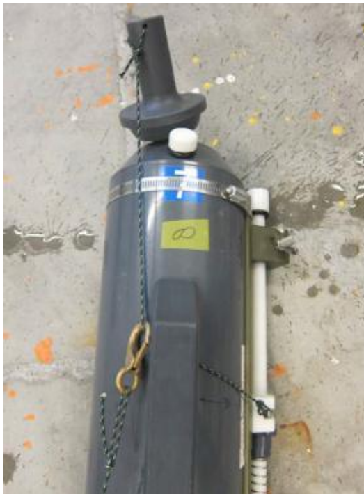
Figure 2: Correct set up for Niskin bottle deployment
