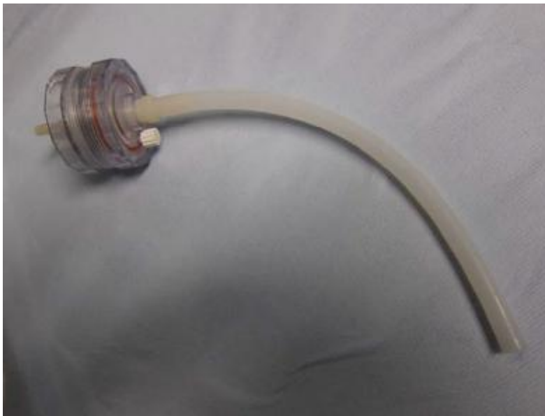
Figure 4: Set up of DOC filtration system for marine sampling, to be connected directly to a Niskin bottle
